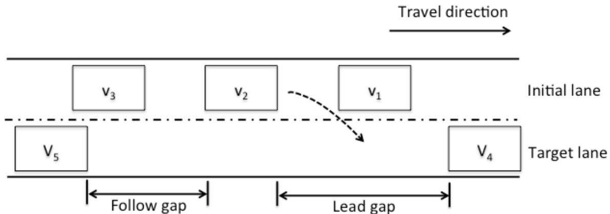
Figure 1 A typical lane changing schematic
